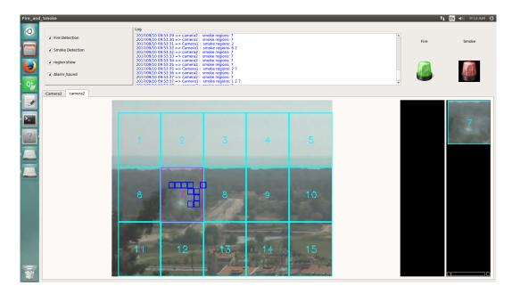
This application is successfully tested as fire  $\mathring{\sigma}$  smoke detector in real condition at Department of Environment of Iran fire extinguisher maneuver in Ilam state. The Software had been running since 2 hours before maneuver started without any false alarm, and when smoke started, it began to send an alert in real-time immediately.
