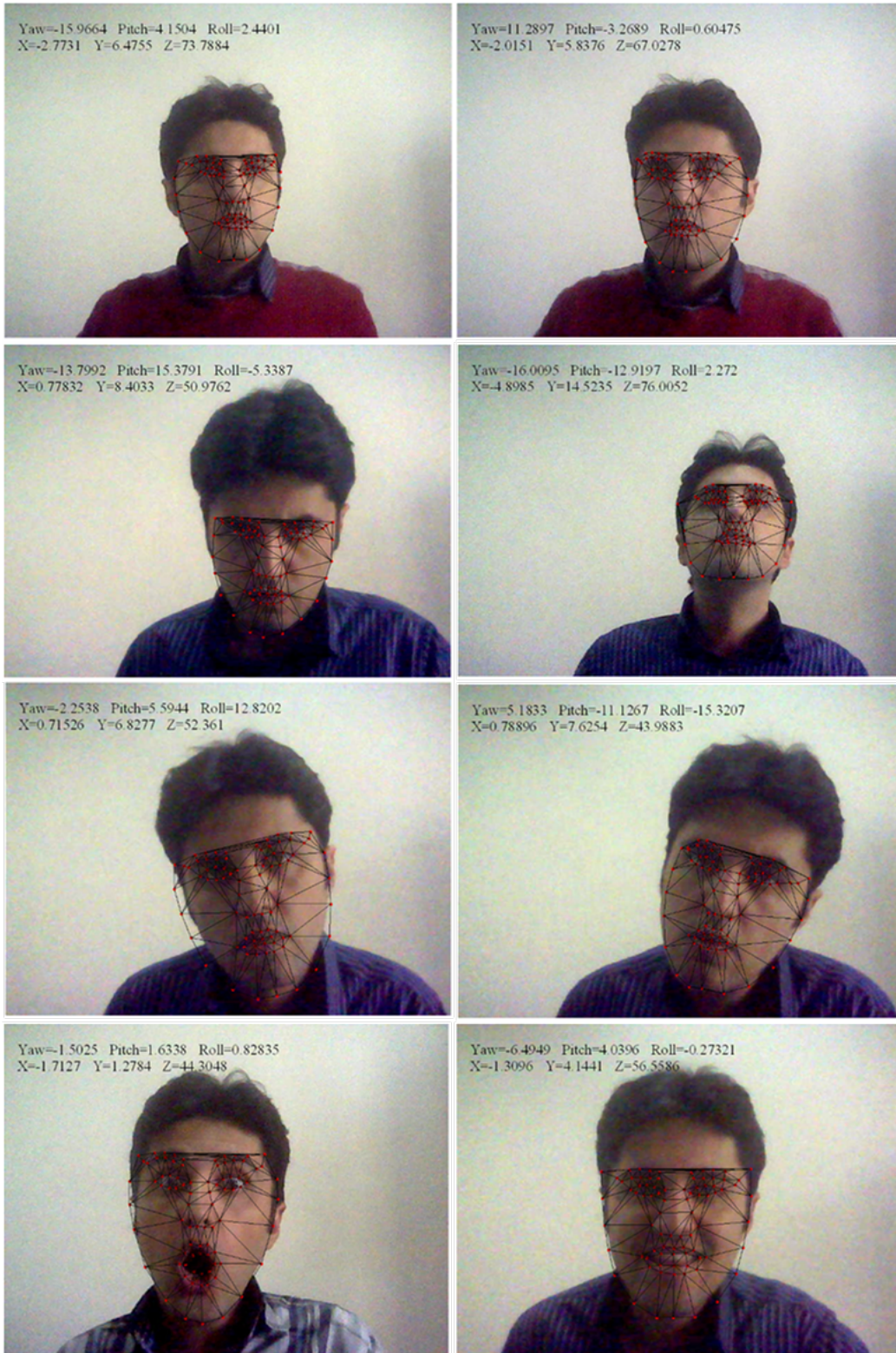
Fig5 Some fitting process results by knowing intrinsic camera parameters
